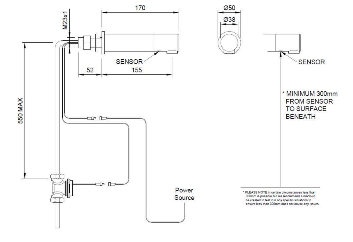
PANEL MOUNTED ELECTRONIC INFRARED TAP DB400C / DB400S / DB400-PC / DB425C / DB425S / DB425-PC
