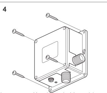
Screw control box in a suitable position under the basin making sure flexihose and control cable can reach.
